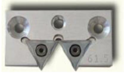
The carbide inserts must be carefully installed in order to insure that the correct cutting angle is maintained. The top of the insert holder pocket is milled at the correct angle to properly align the carbide inserts for an 8-strip, 6-strip, 5-strip or 4-strip rod depending on which cutter head you are using. When you install a set of carbide inserts make sure the top of the inserts are parallel to the insert pocket when they are screwed down.
